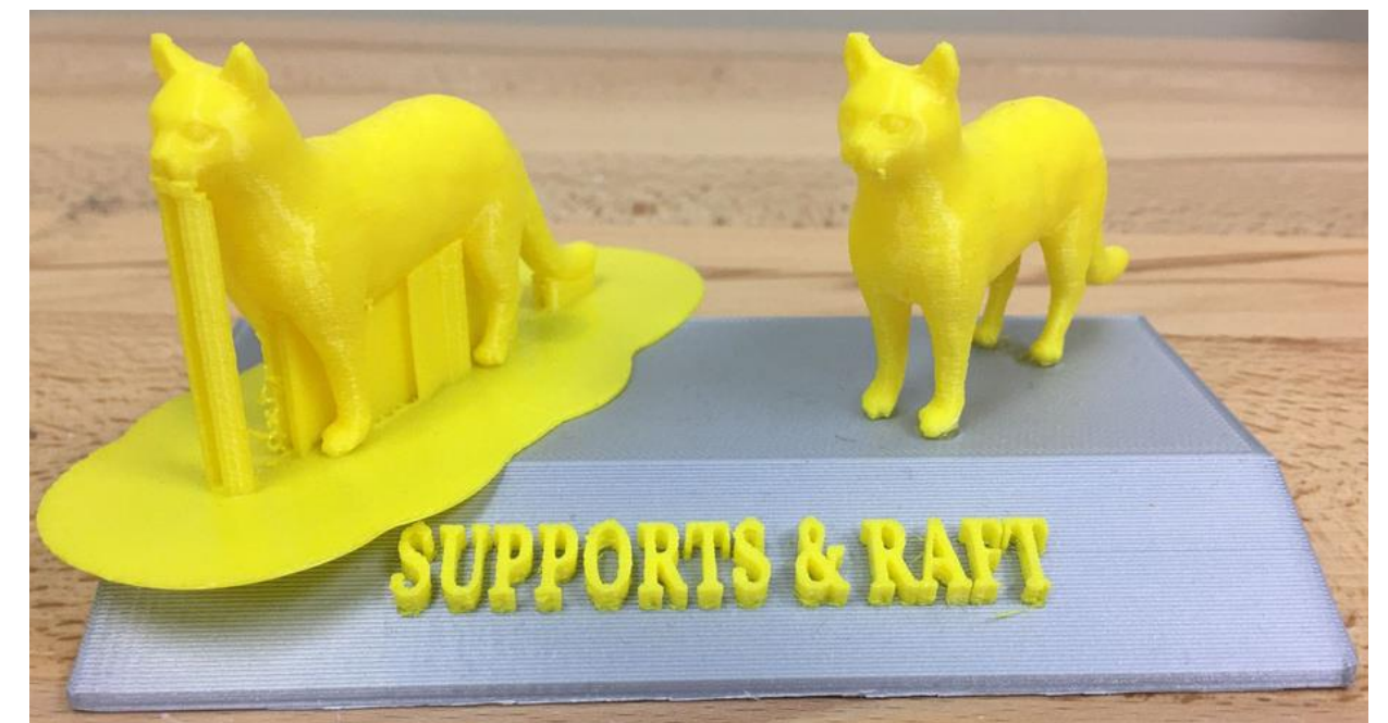
Before and After: Model printed using supports.
